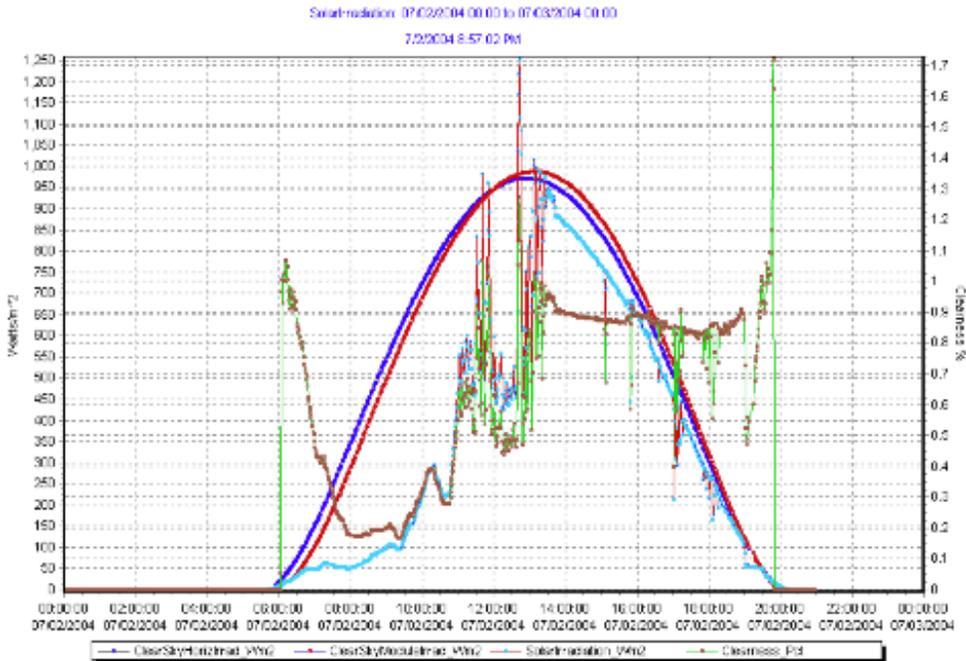
**Solar Irradiance (in green) that Same Day:** Corroborating clouding impacts 11 am – to 1 pm, sunshine drops well under theoretical maximum 1,000 watts/m<sup>2</sup> in same period. For more on Monocrystalline PV1 see our [rooftop performance graph series](#).
