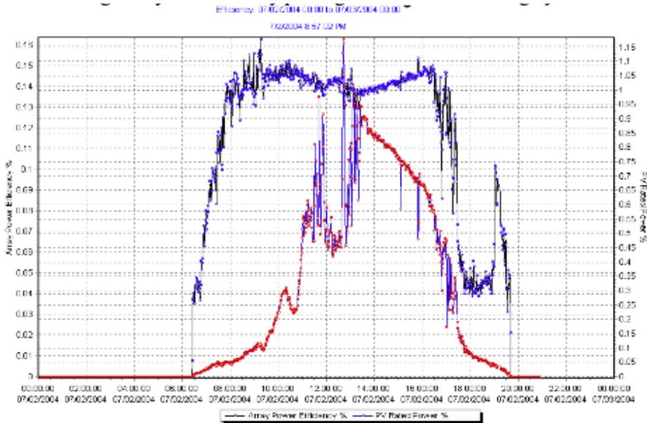
**Sample Array Efficiency & Power over a Day, below:** On a sample day roof mono PV 1 @ 14% module Efficiency was seen to outperform and do well 8 am – to 5 pm. While overall Efficiency (in blue) maintains a desirably flattened, broad parabola, Power output (in red) was more negatively influenced by the passing cloud cover from roughly 11 am – to 1 pm. Cloudy weather can have very sizably impact on PV:
