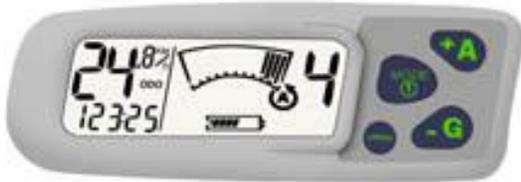
Power-Assist controls 4 assistance levels. An analog display for power from battery.
